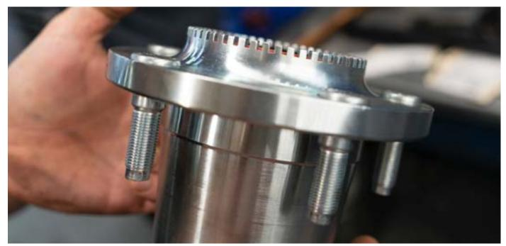
Figure 20. (Seal 0.120-0.160" from top of ABS teeth)
